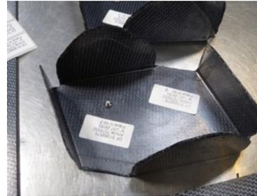
Thermoplastic fuselage clip for Airbus A350. Source: CW
