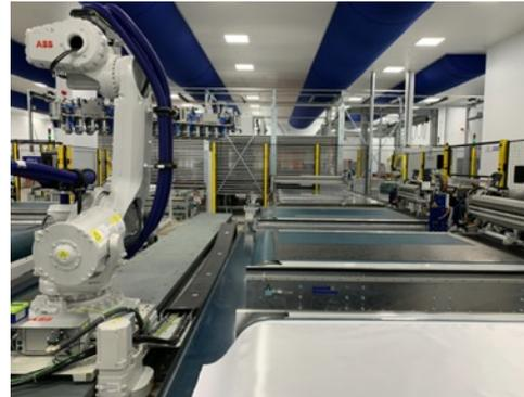
Automated cutting table line at Spirit AeroSystems (Prestwick) for A320 spoiler production. Source: CW
