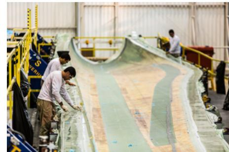
Wind blade layup with balsa core and glass fiber. Source: Aeris Wind Energy
