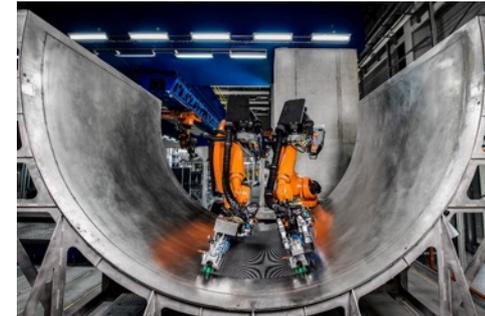
ZLP's autonomous work cell uses an AI-driven work cell to lay up a composite fuselage panel. Source: ZLP Augsburg, DLR
