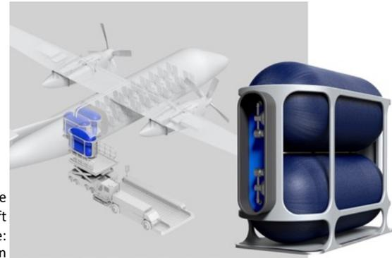
Universal Hydrogen pressure vessel module for aircraft hydrogen storage. Source: Universal Hydrogen
