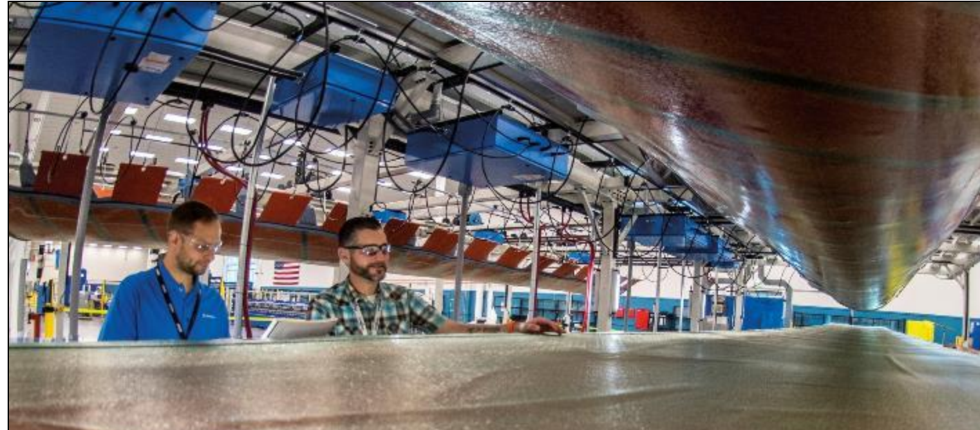
Temper's debulking system shown installed at Boeings West Jordon Facility in the fabrication of 787 rear elevators
